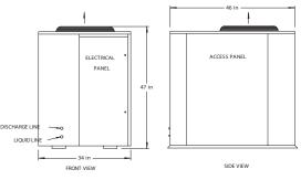
OC Refrigerant Connections: Discharge Line- 3/4", Liquid Line- 1/2"
