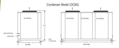
OC Refrigerant Connections: Discharge Line- 7/8", Liquid Line- 5/8"
